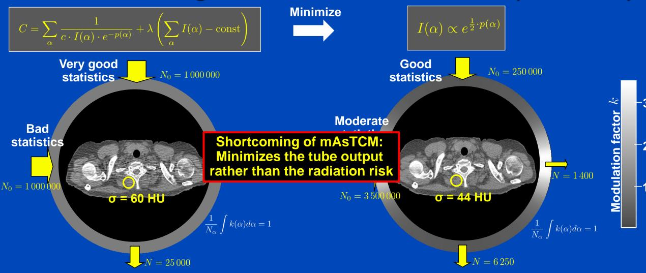
Constant tube current: High, inhomogeneous noise
