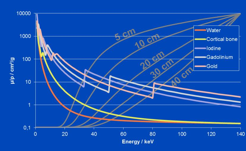
Gray curves: 120 kV water transmission on a non-logarithmic ordinate individually normalized to 1 at 140 keV.
