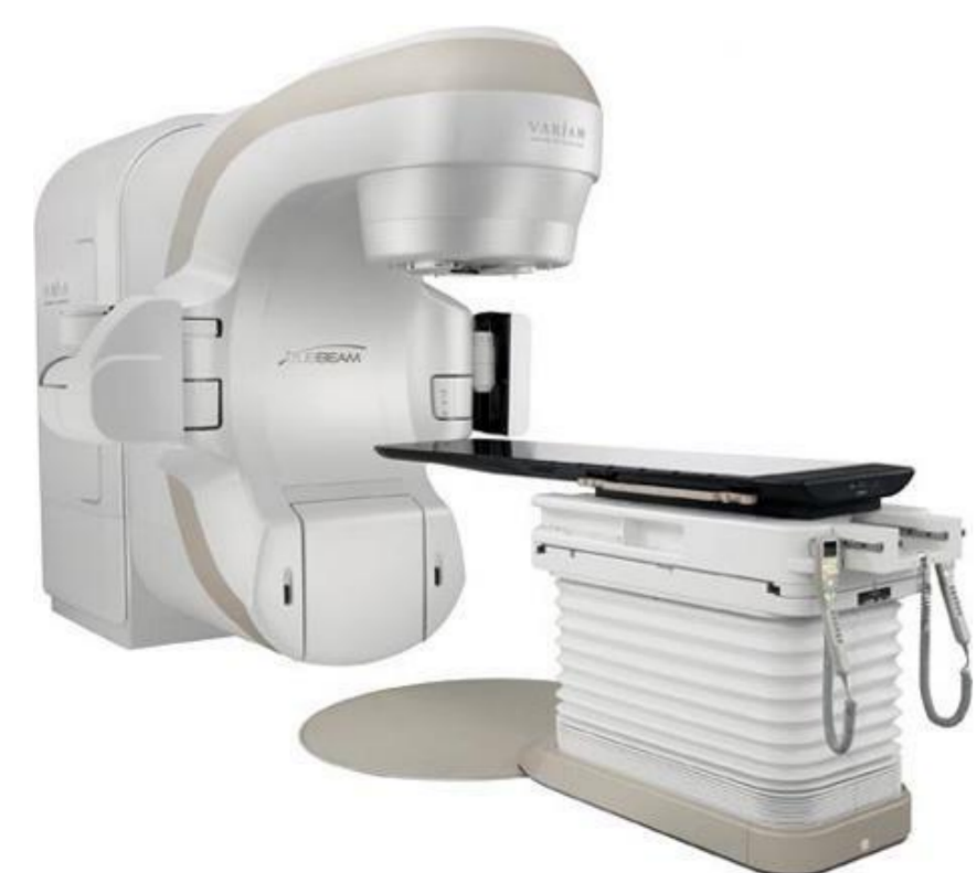
Figure 2: Varian TrueBeam™ geometry: R_F = 100 cm, R_{FD} = 150 cm, N_{360} = 656 projections per full rotation, shifted detector, 1024 \times 768 detector pixels of size 0.388 \times 0.388 mm 2 , t_{\text{rot}} = 60 s rotation time
