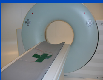
Fig. 3. Placement of the antennas above the CT table. The test persons rest on fully clothed directly above the antennas.
